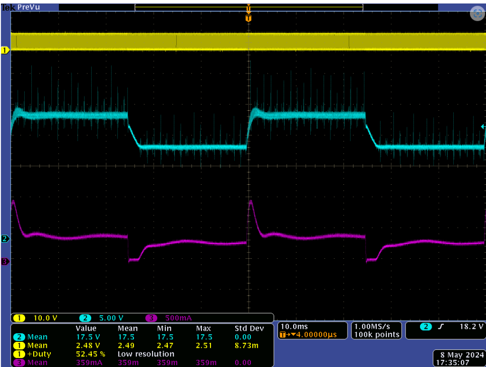
Figure 5.1: Open Loop Voltage and Current @ 10V input
